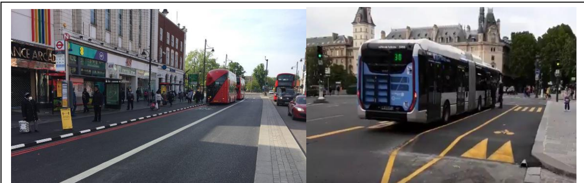
Temporary measures to support public transport –repurposing a traffic lane for additional bus stop queuing and cycle routes.
